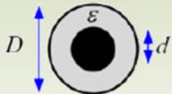
$Z(\Omega) = (138/\sqrt{\epsilon}) \log(D/d)$<br>66% (PE) à 80% (semi-aéré) |
